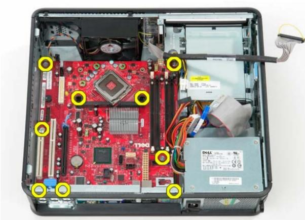
*Figure 5.5.5.6 Motherboard Screws*
