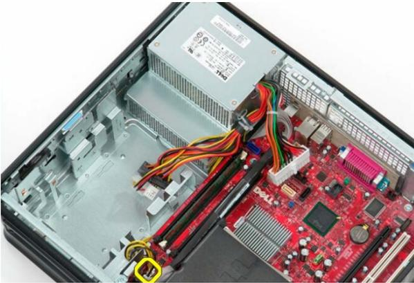
*Figure 5.5.4.2 Power Supply Processor Connector*
