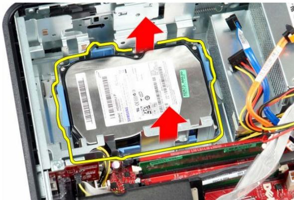
*Figure 5.5.3.3 Hard Drive Removal*
