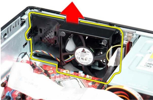
*Figure 5.5.7.3 Fan Removal*
