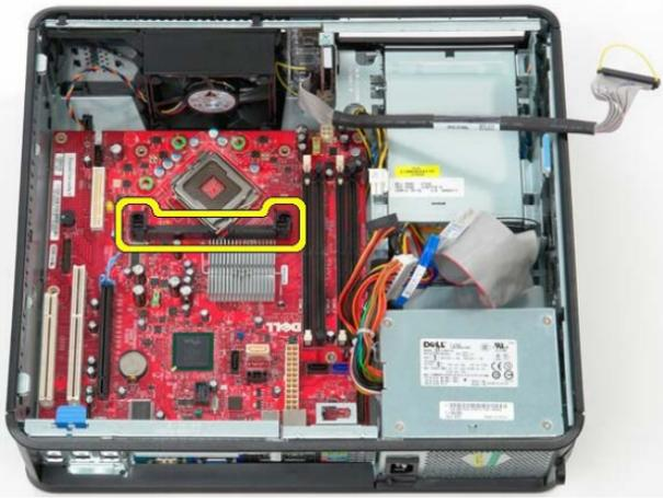
*Figure 5.5.5.7 Motherboard Assembly Bracket*
