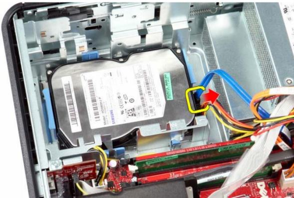
*Figure 5.5.3.1 Hard Drive Connection*
