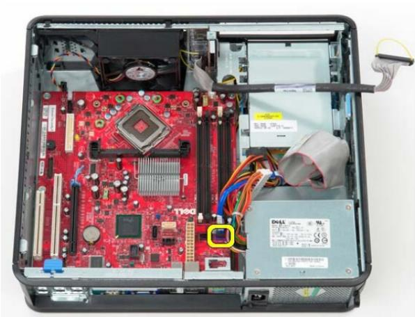
*Figure 5.5.5.4 Hard Drive Connection*
