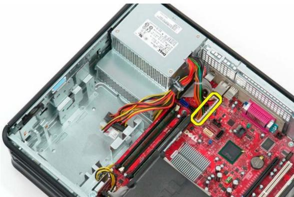
*Figure 5.5.4.1 Power Supply Main Connector*
