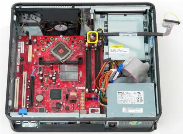
*Figure 5.5.5.5 Processor Connection*
