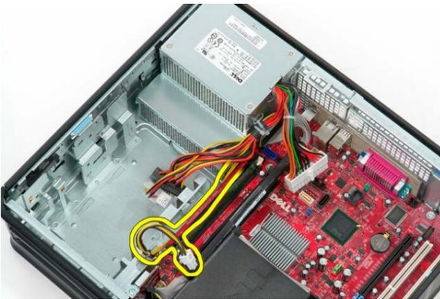
*Figure 5.5.4.3 Power Supply Motherboard Connector*
