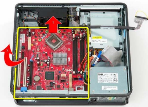
*Figure 5.5.5.8 Motherboard Removal*
