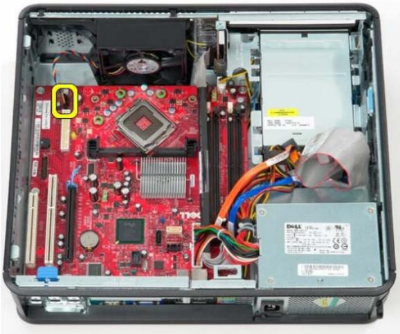
*Figure 5.5.5.1 Fan Connection*
